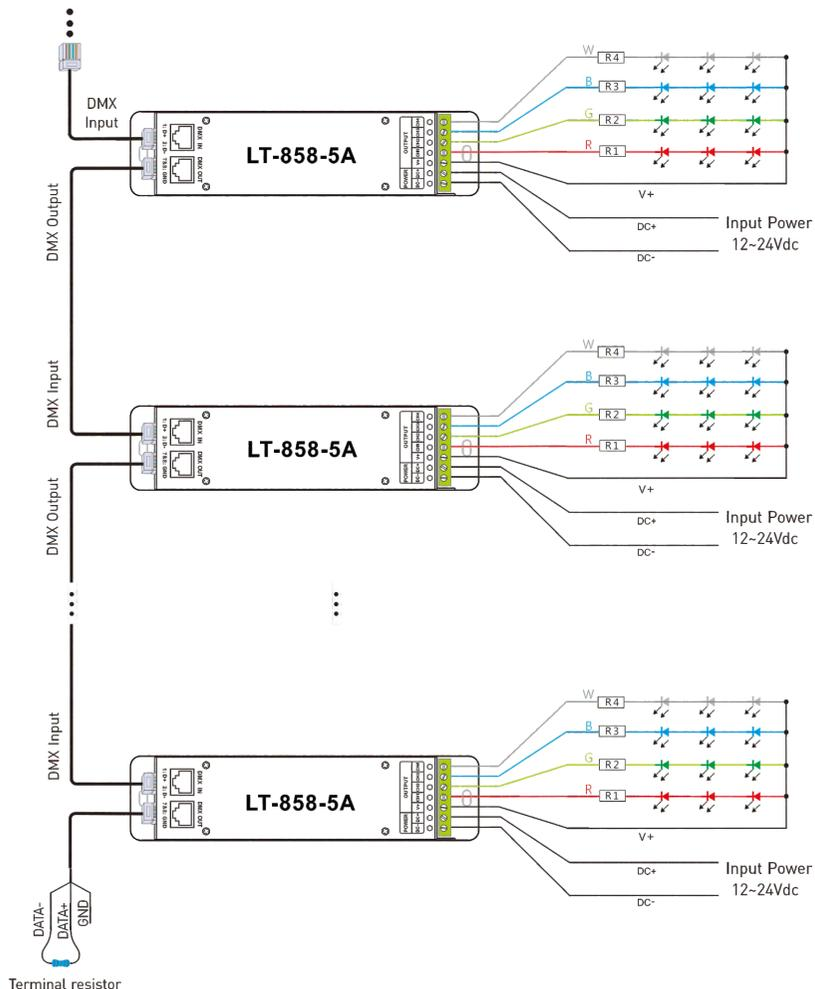
\* If the recoil effect occurs because of longer signal line or bad line quality, please try to connect 0.25W 90-120Ω terminal resistor at the end of each line.
